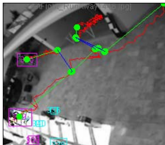
Fig. 3. A low-level procedure discriminates trajectories (red lines) of objects (violet rectangles) and moments of their interactions (green circle marks).
