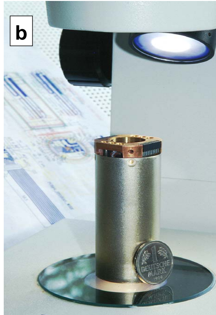
Fig 10. Laboratory Integrated receiver (a). Photographs of exchangeable receiving head (length 76 mm and diameter 32 mm); the input aperture and connectors are seen on the top (b).
