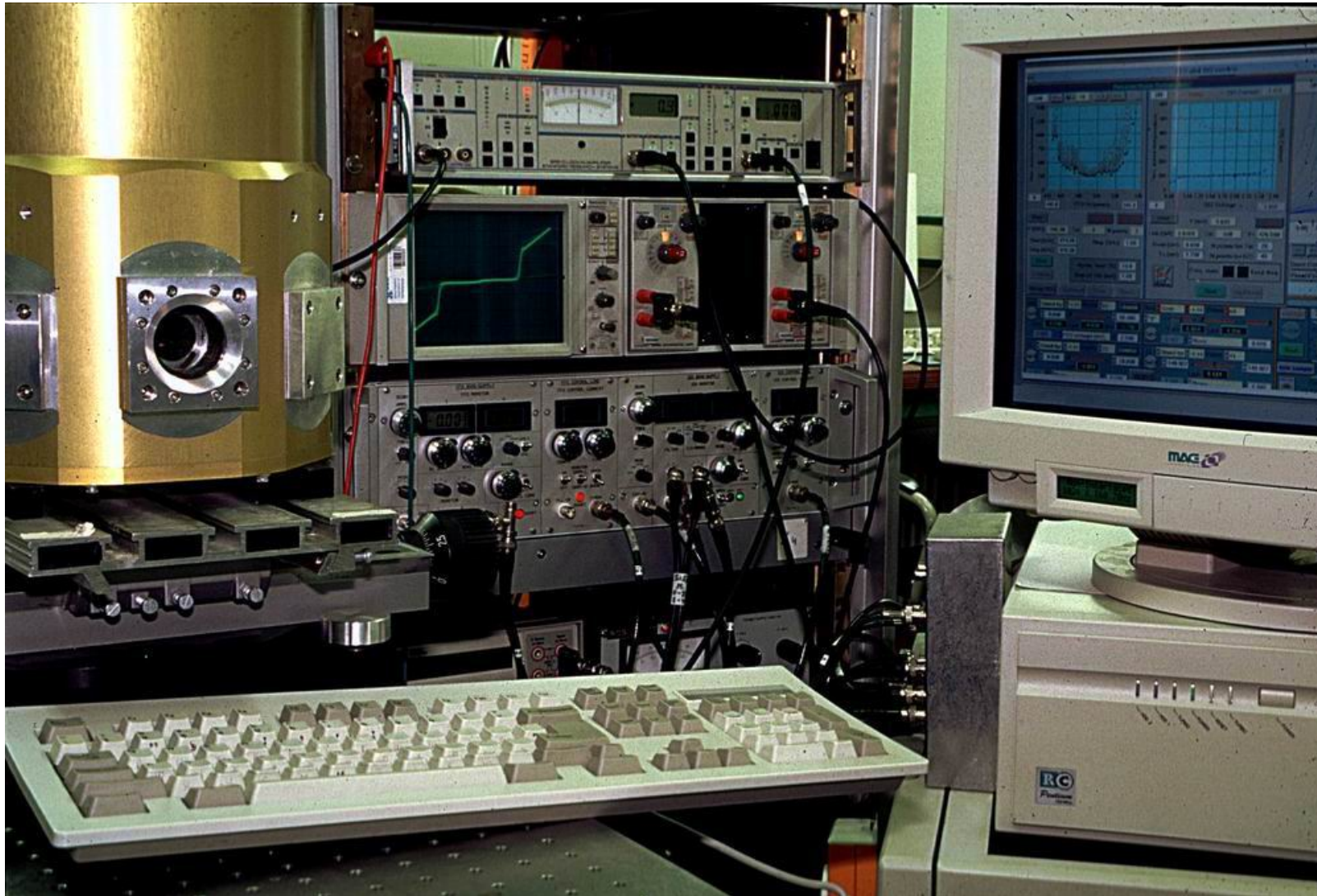
Fig 9. Photo of the experimental set-up controlled with IRTECON system: quasi-optical cryostat at the left, bias supply unit in the center (at the background) and data display at the right.
