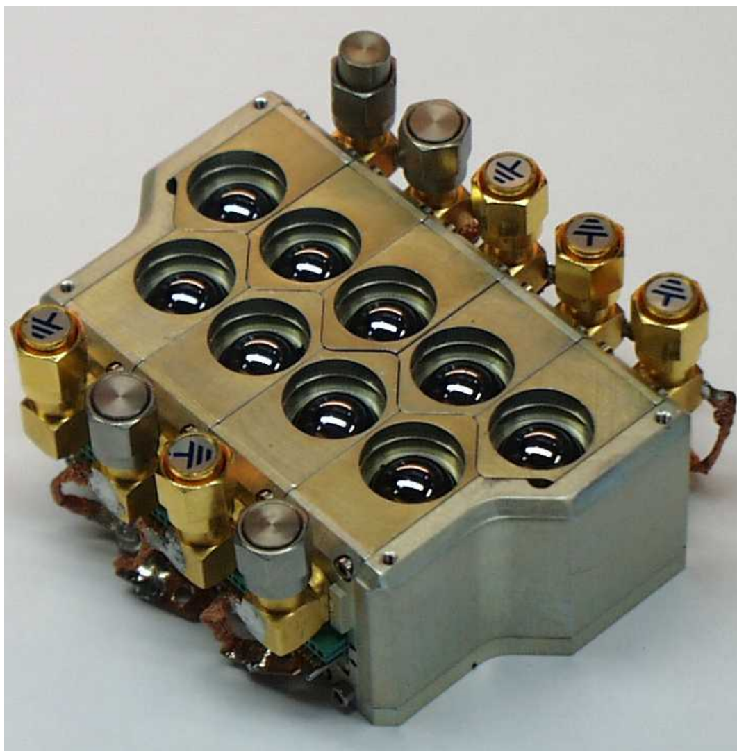
Fig 8. Nine-pixel imaging array receiver block. Each pixel is an independent integrated receiver with its own internal local oscillator. The array mount is shown from the side of its input microwave lenses.
